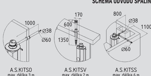
SCHÉMA ODVODOU SPALIN
